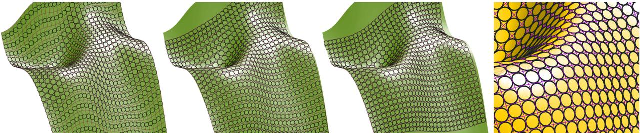
Figure 9: The converging (contracting) grid is perfectly suitable for a circular pattern that covers the surface. Left: Starting position, right (yellowish): converged grid.
