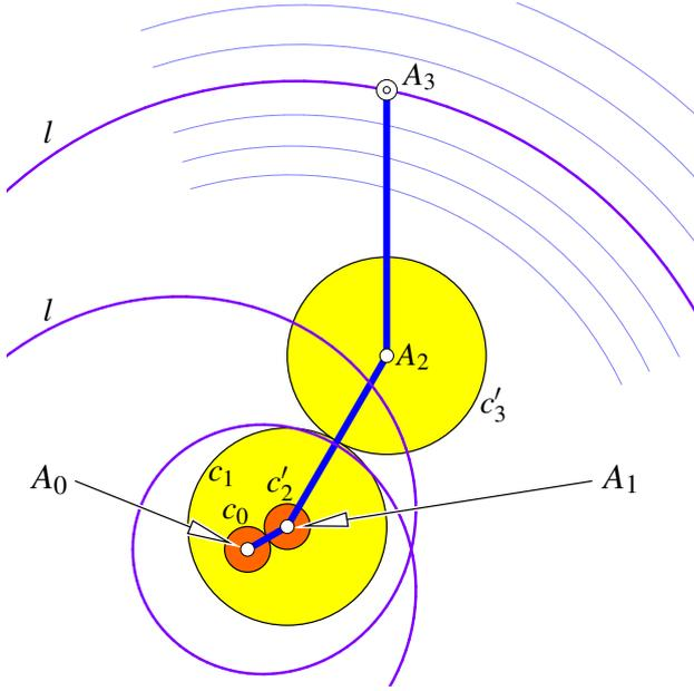
Figure 7: The top views of  $\mathcal{M}$ 's parameter curves generated either with rolling circles or by an open three-legged kinematic chain.
