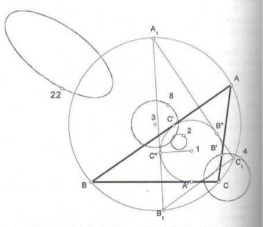
Fig. 9.9 Circular orbits of centers 2, 4 and 8; noncircular orbit of center 22
